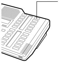
Memory buttons are the buttons with labels other than line or Handsfree buttons. Memory buttons store telephone numbers or feature codes to give you one-touch dialling or feature activation. You can change the function of a memory button by programming it with a new number or feature.
